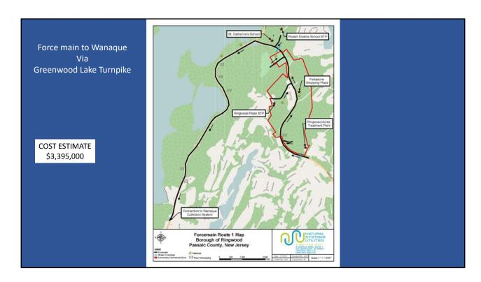
Ideally, a solution to all of the existing and potential problems with these various treatment and discharge facilities might be to combine them and construct a low pressure sewer force main with grinder pumps and connect it to the Wanaque Valley Regional Treatment Plant through the Wanaque local sewer system
